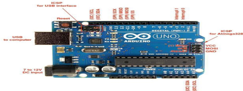
Figure2: Arduino board
