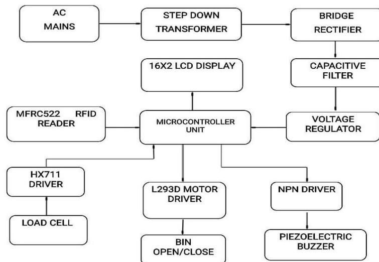
**Fig.1 Block diagram for RFID**
