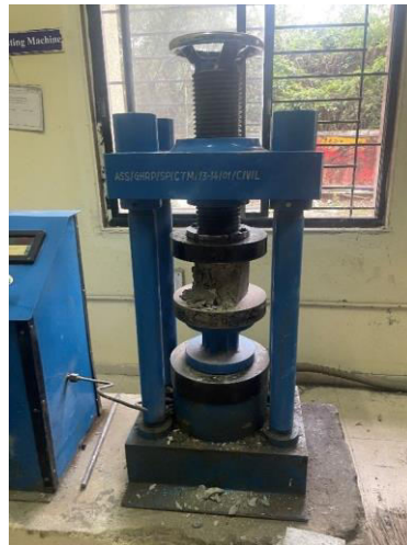
Fig. 10 Testing of Cubes
