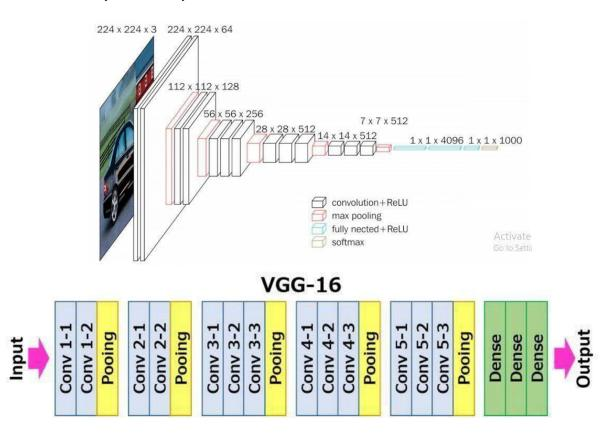
The "16" in VGG16 refers to the 16 layers with learnable weights, comprising 13 convolutional layers and 5 max-pooling layers, totaling 21 layers. It accepts input images of size 224x224 with 3 RGB channels. VGG16 simplifies
