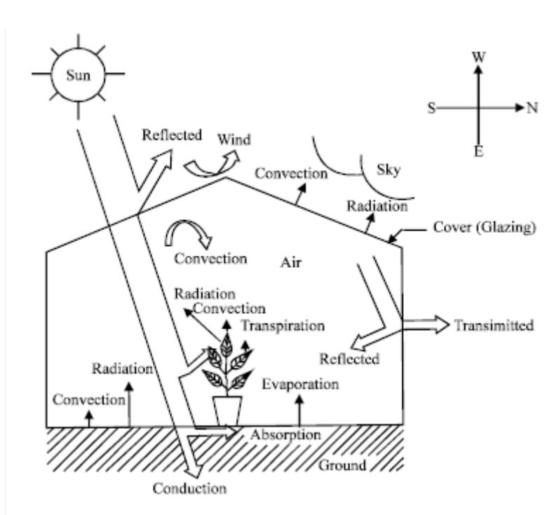
Fig. 3: Energy flow processes in greenhouse system
