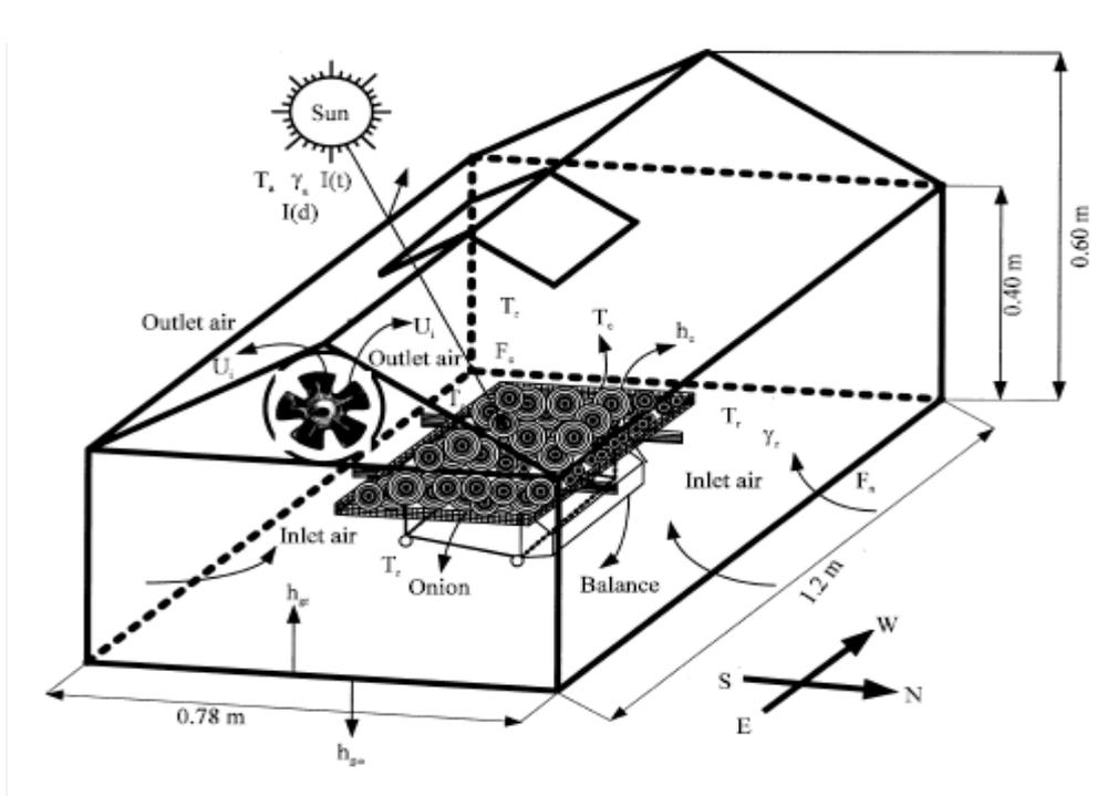
Fig. 4: Schematic view of greenhouse dryer
