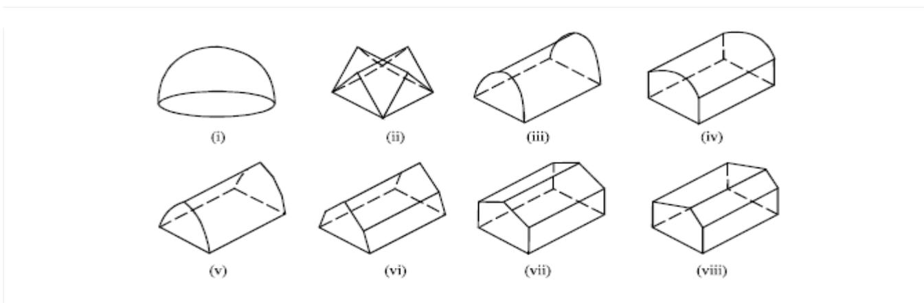
Fig. 5: Classification of greenhouse on the basis of shape; (i) Spherical dome, (ii) Hyperbolic paraboloid, (iii) Quonset, (iv) Modified Quonset, (v) Gothic arch, (vi) Mansard roof, (vii) Evenspan and (viii) Unevenspan
