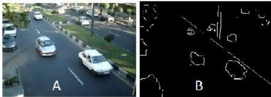
Figure 3. A: Original image B: Edge detection result
