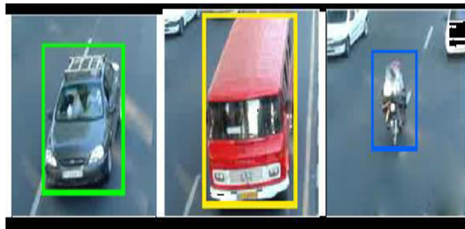
Figure 5. Vehicle classification-coloured bounding boxes
