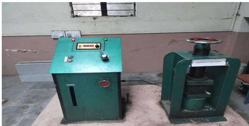
Fig -4: Testing on concrete cube on (CTM)
