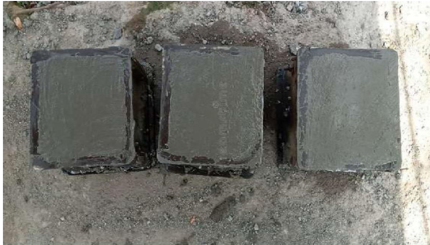
Fig -2: Concrete cube keep for 24 hrs
