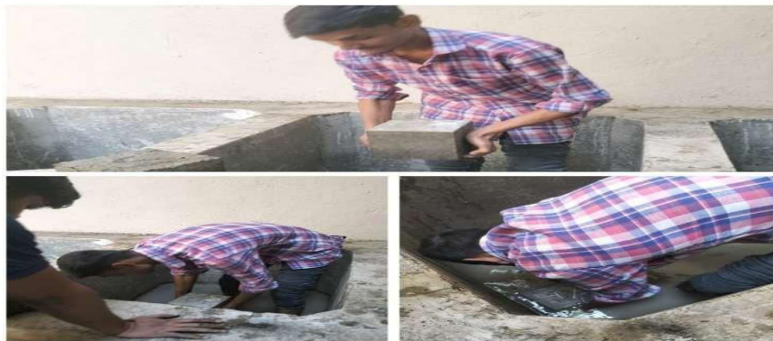
Fig -3: Concrete cube for curing for( 7 days, 14 days, and 28days)
