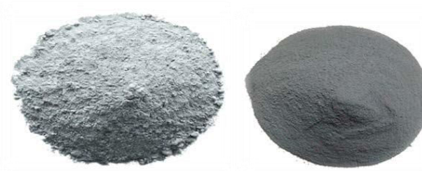
Figure 1. Fly Ash (Left) & Silica Fume (Right) Supplement Materials
