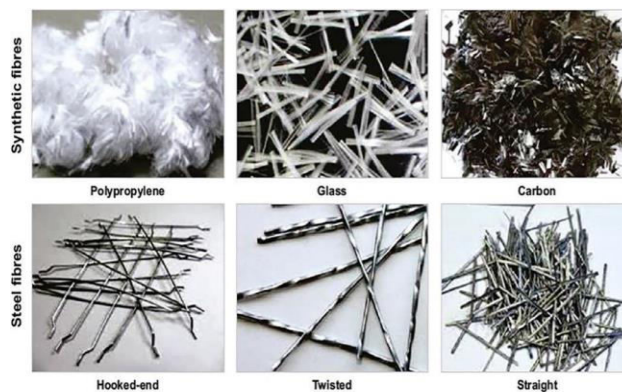
Figure 4. Fibers commonly used to Reinforce Concrete
