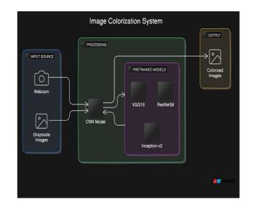
The Image Colorization System is designed to transform grayscale images or live video feeds into vibrant, colorized outputs using deep learning techniques. Its architecture is composed of three major modules: Input Source, Processing, and Output.
