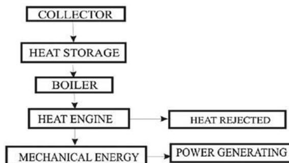
Fig. 3 Schematic diagram of a solar thermal conversion system
