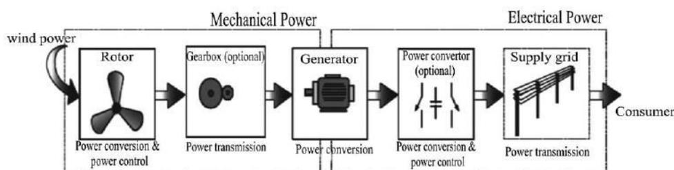
Fig. Conversion from wind power to electrical power in a wind turbine
