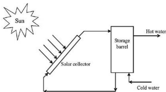
Fig. 2. A typical domestic-scale solar water heater
