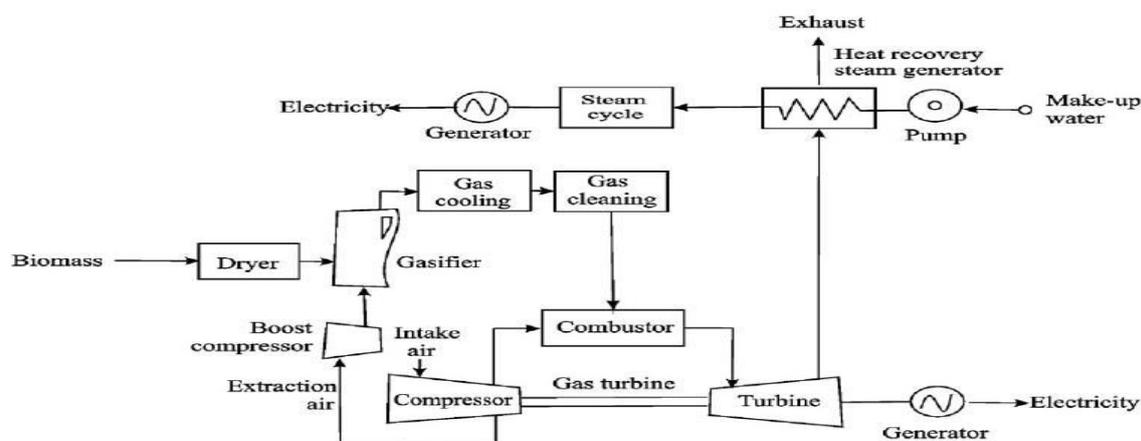
Fig. A biomass-gasifier/gas turbine combined cycle
