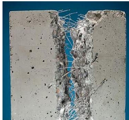
Figure no. 1 ;Steel fiber-reinforced concrete
