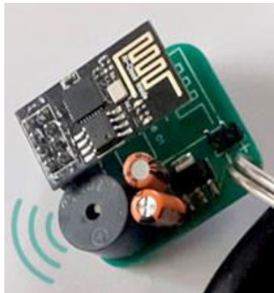
Fig 4. Customised PCB of Tag
