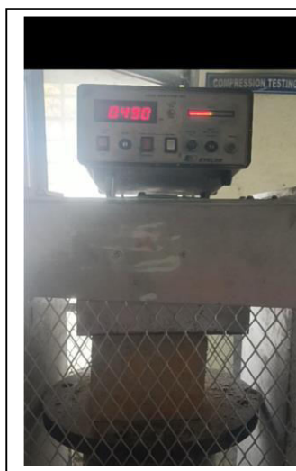
Figure 3. Compressive Strength testing machine (CTM).
