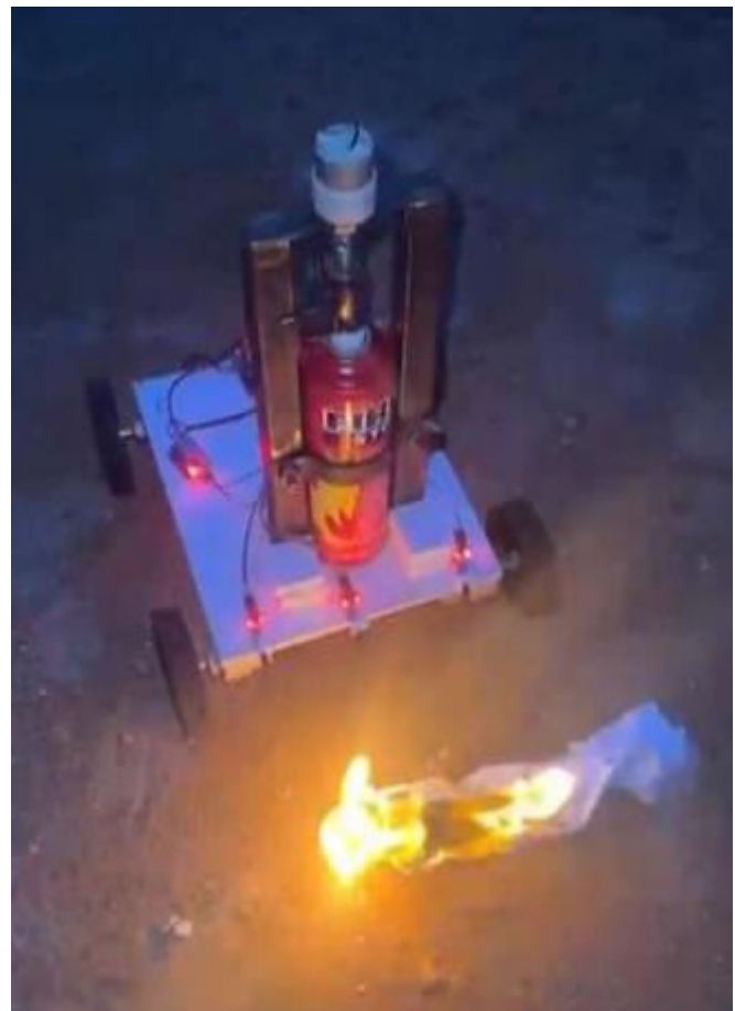
Fig2. Automated Sensor Based Fire Extinguisher Mounted On AGV
