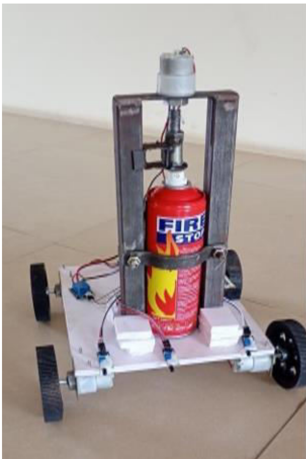
Fig2. Automated Sensor Based Fire Extinguisher Mounted On AGV
