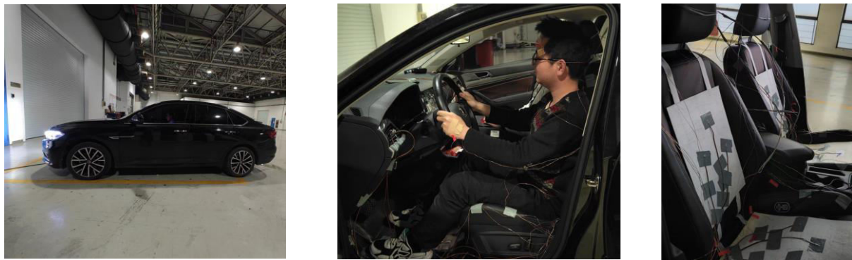
Figure 1: (a) Experiment vehicle. (b) Experiment subject. (c) Measured points in the cabin.
