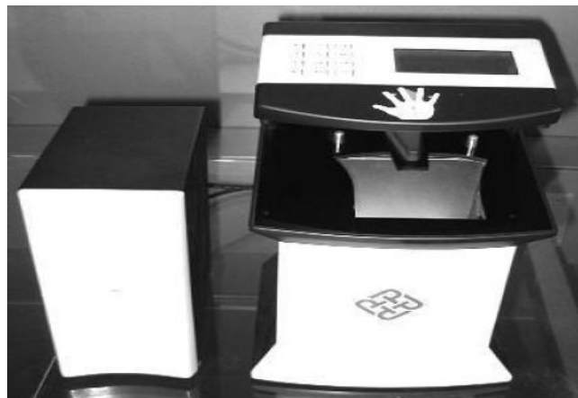
Fig -4: CCD-based palmprint scanner
