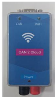
Fig 2. CAN to Wi-Fi Module
