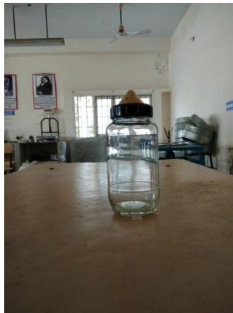
Figure 1: Pycnometer used for finding out Specific Gravity of materials.
