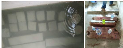
Figure 3: Curing of Specimen ;
