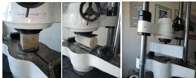
Figure 5 : Strength Tests on Specimens.
