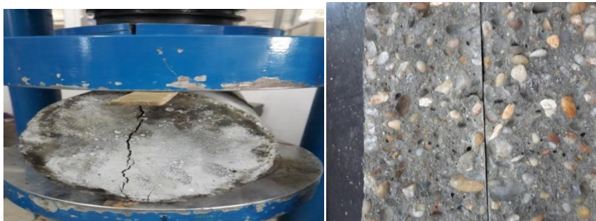
Fig. 7 split tensile test for cylinder
