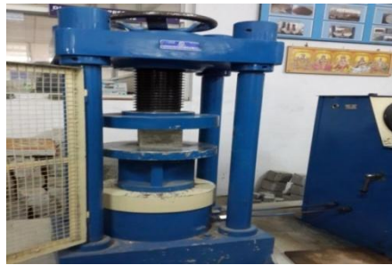
Fig. 6 Compression test for cube
