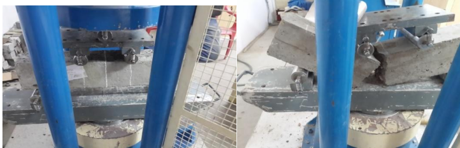
Fig.8 Flexural test for beam
