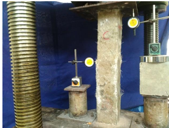
Fig 5.5. Testing of GFRP wrapped conventional column
