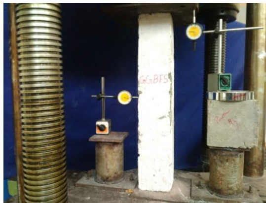
Fig 5.3 Testing of BACILLUS Bacteria replaced R.C column
