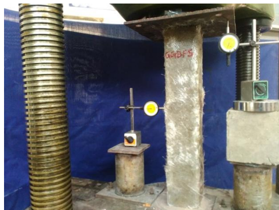
Fig 5.4 Testing of GFRP wrapped BACILLUS Bacteria column
