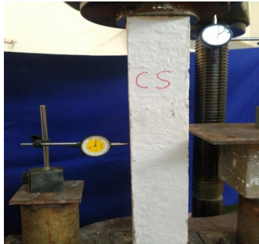
Fig 5.2. Testing of conventional R.C column
