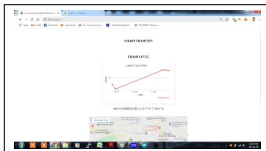
Fig. 9: Webpage displaying the dynamic graph reading the dustbin readings
