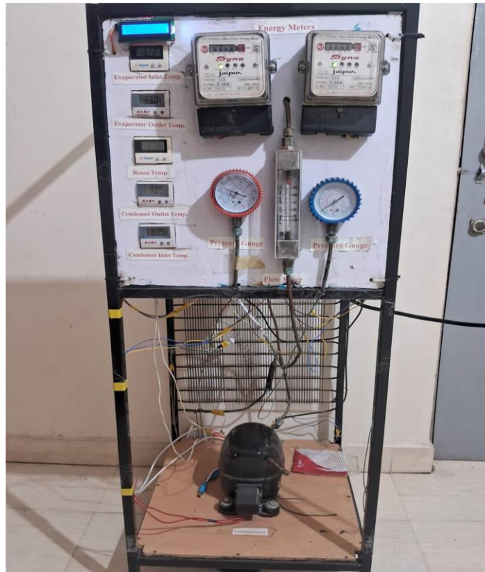
Fig. 2. Working model in Refrigeration System Fault Detection By Using Machine Learning
