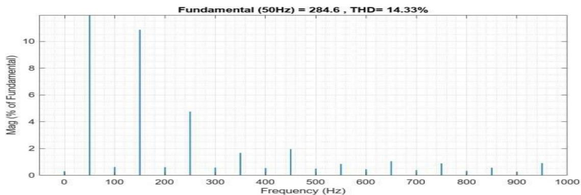
Fig 6. THD output with R load of 15-level
