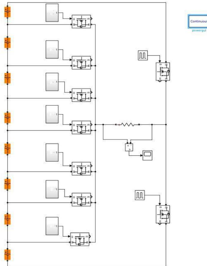
Fig3.Circuit diagram of CHB 15-level inverter with reduced switches with R load
