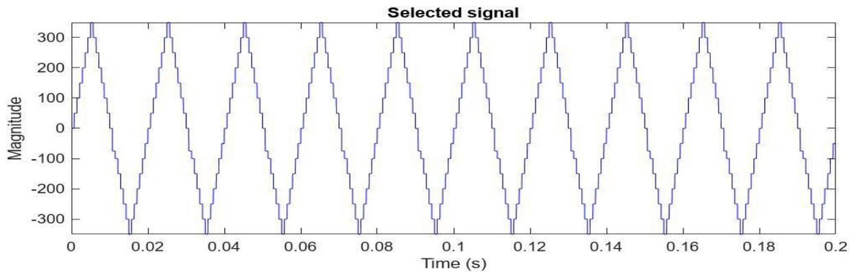
Fig. 5 .Simulation output of 15-level inverter
