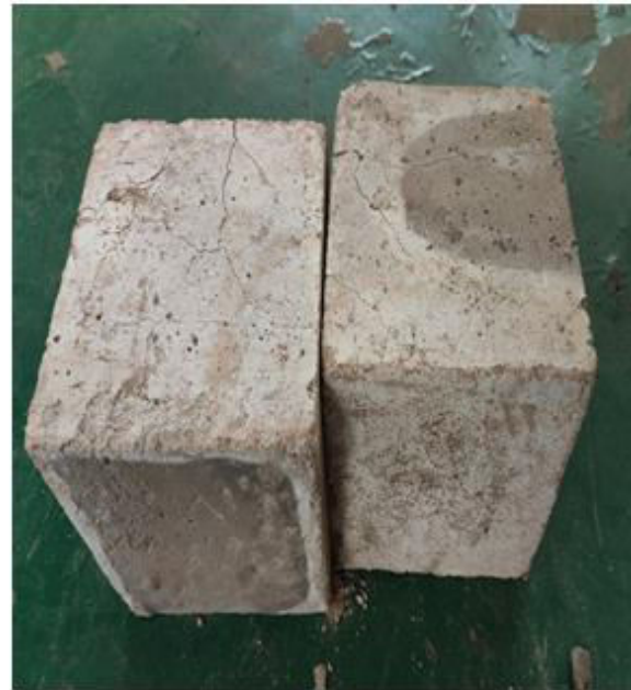
Figure 6 Cubes removed from HTF
