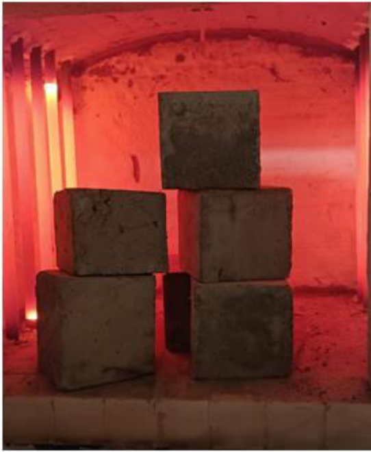
Figure 5 Cubes kept in HTF in 900 °C
