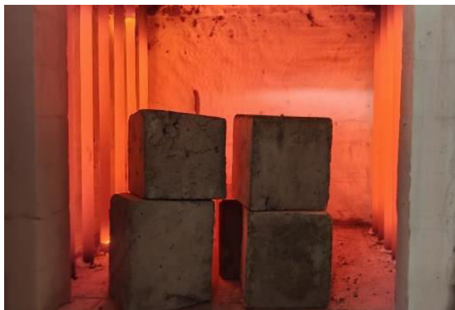
Figure 1 Temperature furnace at 900 °C
