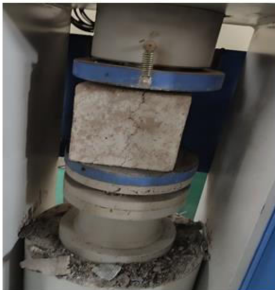
Figure 7 Compression test after removed from HTF
