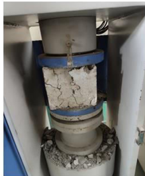
Figure 7 Compression test after removed from HTF
