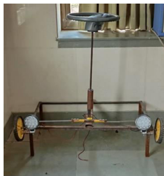
Fig.3.1 Working model of movable headlight mechanism with headlight.
