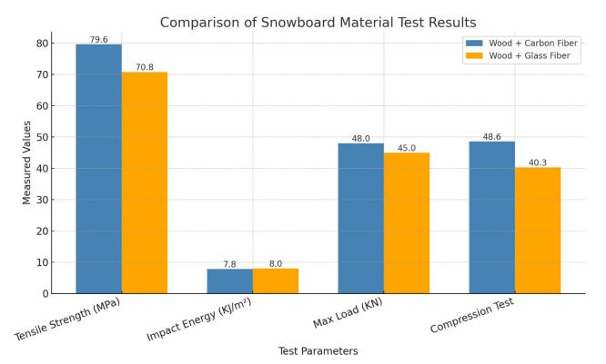
In this Fig, The graph shows visually compares the mechanical properties of Wood + Carbon Fiber and Wood + Glass Fiber composites based on test results. It includes four key parameters: Tensile Strength, Impact Energy, Maximum Load, and Compression Strength.
