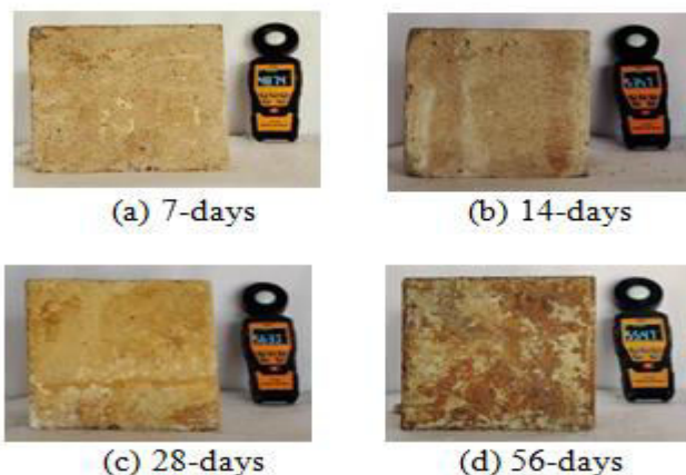
Figure 3: Hydrochloric acid immersion at 5% concentration after (a) 7 days, (b) 14 days, (c) 28 days, and (d) 56 days.
