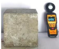
Figure 2: Control sample before immersion in chemicals.
