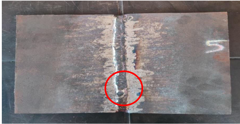
Fig 4.1 visual inspection result of test sample 5.
