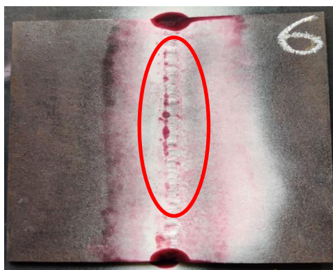
Fig 4.3 test sample which showing falls indications.
