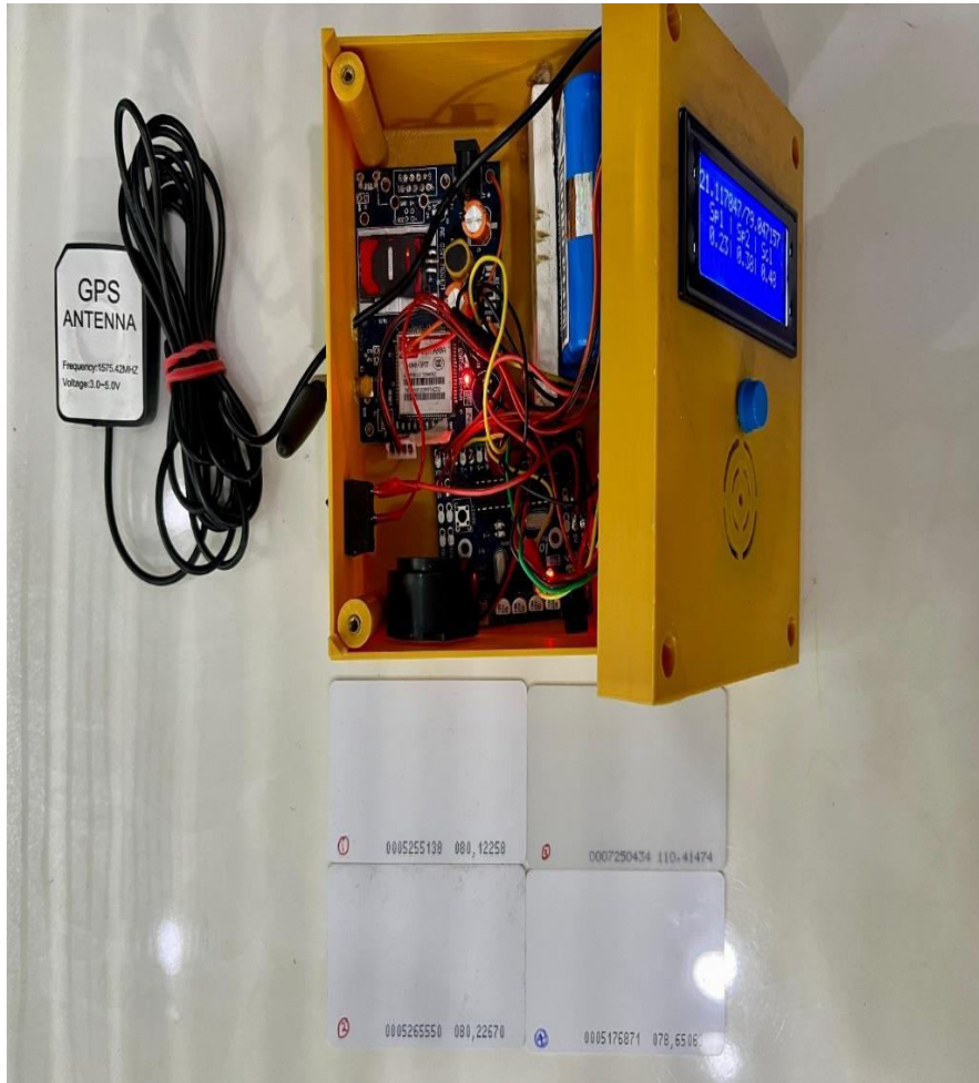
Fig(iii) Encloser Box with System Hardware Assembly and Battery Power Source.
